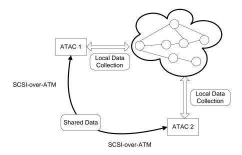
RAID7 allows multiple hosts to simultaneously link to the same data. This feature is efficient. One host is not required to copy the data to deliver it to another, or to engage in data collection, which allows the host's CPU to be devoted to processing data. Costly mainframes are not required for maximum data handling.
